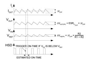
Figure 2. MIC24051 Control Loop Timing
