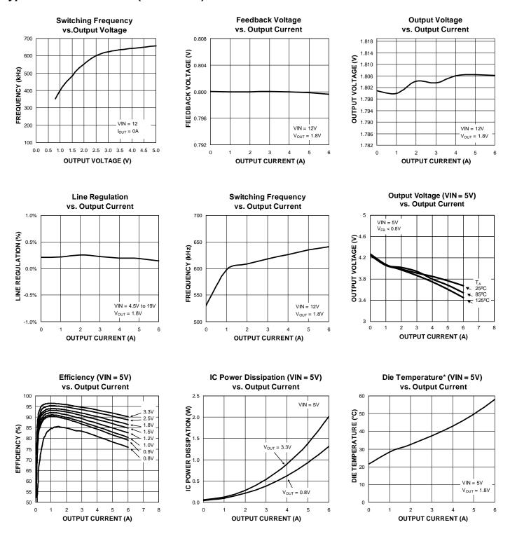
**Die Temperature\***: The temperature measurement was taken at the hottest point on the MIC24051 case mounted on a 5 square inch 4 layer, 0.62", FR-4 PCB with 2oz finish copper weight per layer, see Thermal Measurement section. Actual results will depend upon the size of the PCB, ambient temperature and proximity to other heat emitting components.
