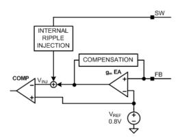
Figure 9. Internal Ripple Injection
