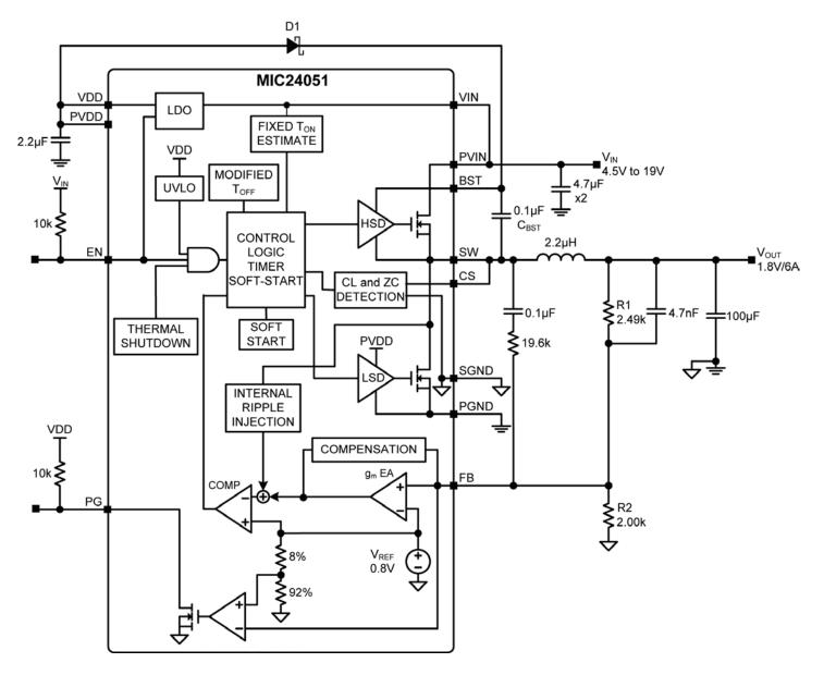
Figure 1. MIC24051 Block Diagram
