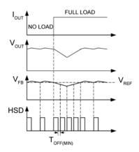
Figure 3. MIC24051 Load Transient Response
