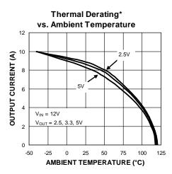
**Die Temperature\***: The temperature measurement was taken at the hottest point on the MIC24051 case mounted on a 5 square inch 4 layer, 0.62", FR-4 PCB with 2oz finish copper weight per layer, see Thermal Measurement section. Actual results will depend upon the size of the PCB, ambient temperature and proximity to other heat emitting components.
