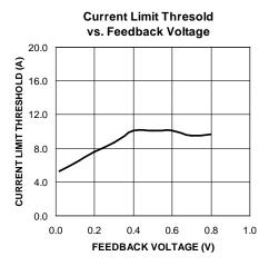
Figure 4. MIC24051 Current-Limit Foldback Characteristic
