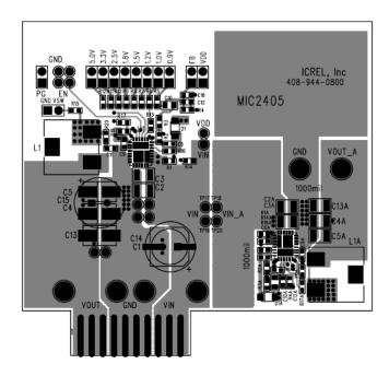
Figure 12. MIC24051 Evaluation Board Top Layer
