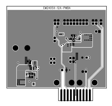
Figure 15. MIC24051 Evaluation Board Bottom Layer
