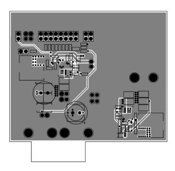
Figure 14. MIC24051 Evaluation Board Mid-Layer 2
