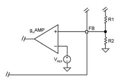
Figure 8. Voltage-Divider Configuration
